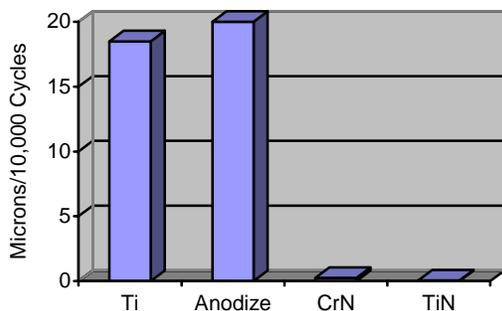
**Figure 3: Abrasive wear rate comparison for untreated and treated Ti (CP)**
