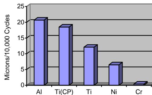
**Figure 1: Abrasive wear rate comparison for untreated alloys (CS-10 wheel).**
