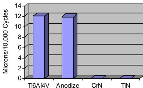
**Figure 4: Abrasive wear rate comparison for untreated and treated Ti-6Al-4V.**
