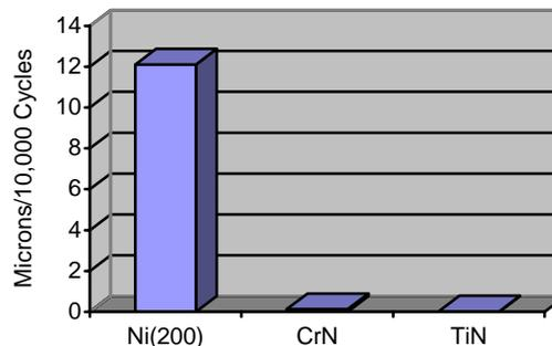
**Figure 5: Abrasive wear rate comparison for untreated and treated Ni-200.**
