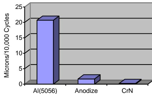
**Figure 2: Abrasive wear rate comparison for untreated and treated Al (5056).**
